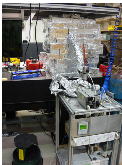
FIGURE 3.7: The oven during the bake out process. The turbo pump and Residual Gas Analyzer (RGA) are mounted on the turbo pump station.
