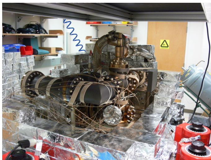
FIGURE 3.6: The oven under construction is prepared for the bake out. The variable AC transformers, heater tapes and thermocouple wires are shown in the picture.
