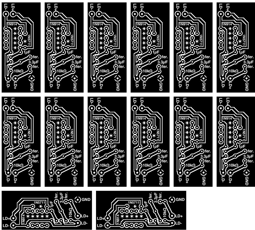
DIODE LASER PROTECTION CIRCUIT
