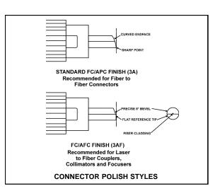
air gap between the fiber and the lens, the backreflection level for the endface of the fiber is about -14dB. This can be reduced to -40dB to -60dB by slant polishing both fiber ends to deflect the backreflected signal.
