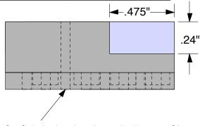
Thru-hole for dowel pin (or small Allen wrench)
