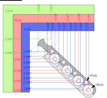
(Dimensions measured from lower left hand corner of cavity body)
